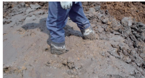
Photo 5 東京湾岸部の沖積粘性土の例 (The Example of Alluvial Clay Distributed around the Tokyo Bay)
