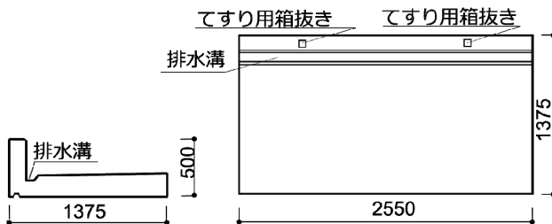
Fig. 5 バルコニー部材の外観 (Appearance of Mock Up)
