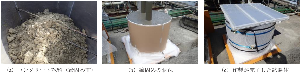
Photo 2 試験体の作製状況 (Preparation of Test)
