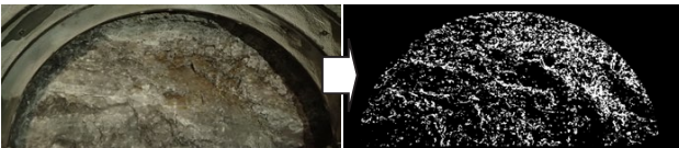
Fig.7 風化変質判定の例 (Example of Weathering Evaluation)
