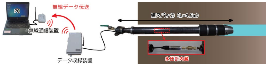
Fig.12 短尺スイリモシステム (Monitoring System of Water Pressure Using Short Boring)
