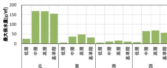
Fig. 5 運用時の各方位高さ毎の結露量 (Dew Condensation in Operation Related to Orientation and Floor Height)
