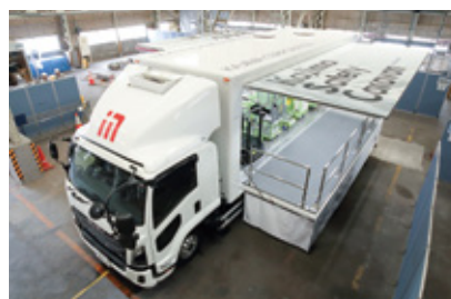
The training vehicle is a mid-sized (11t) truck equipped for nine types of hazard simulation training.
