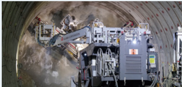
A^CSEL for Tunnel, automated rock bolt installation
